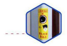
\* Non-touch temperature measuring far away 1-50cm distance, the fastest detection time is less than 0.5 seconds
